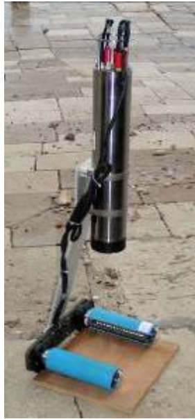
Figure 2. The UVP stand-alone version. The working range of the UVP is 0- 3000 meters and the volume of each image acquired at the frequency of 5 im/s is 1,2 litres. The abundance and size of zooplankton is sorted in situ and visualized onboard.
