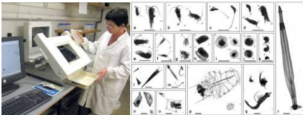
Figure 1: Right: sample recovery from the ZooScan following the digitisation, left: Mediterranean zooplankton ZooScan image.
